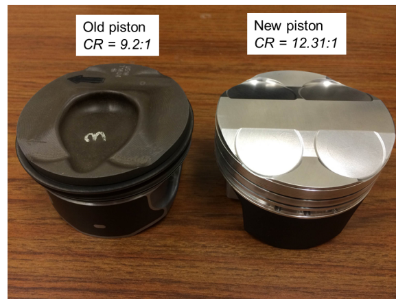
Figure 2.9: Stock and new piston top designs
